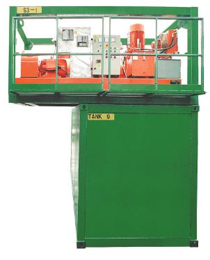
tank so that the whole unit may be transported as a standard type 1CC, 20 foot freight container complete with ISO corner castings.
